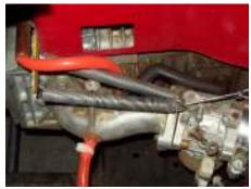
For V-twins and different style carburetors' used on FXS/FXT, the same principle must be used. For example FXS/FXT using Mikuni or the CV style Keihn Carburetors the Slide Spring can count as one return spring and you must have a separate external spring attached as the safety spring.
